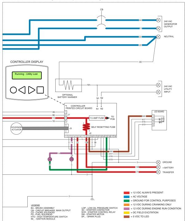
Figure 4. Circuit Condition - Engine Startup and Running
